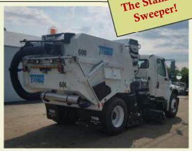
This Tymco 600BAH offers a 6-Yard capacity, Diesel JD 4045T T4 99HP Engine, Stainless Hopper & Housing, Dual Digger RH Tilt Gutter Brooms, High Output Water, Air Purge ASI, PHU Curtain Lifter, and Sweeper Deluge, along with tons of additional features!
