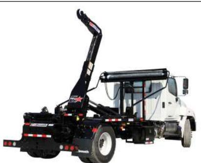
Designed to operate in a variety of applications this hook hoist can be used in the **Waste, Construction, Landscaping & Auto Industries**. The U20-HK & U30-HK models offer benefits through their versatility and dual hook height capabilities.
