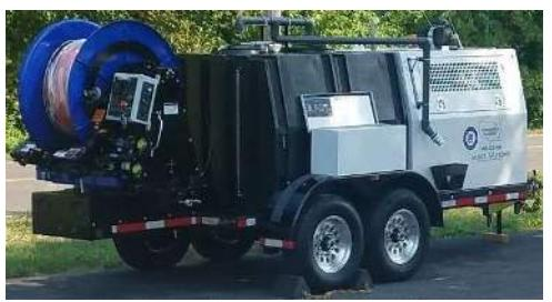
This series of hydro-jet cleaners offer a Ford gas engine and Giant triplex plunger run-dry pump as standard equipment, assuring customers of a vast support network, utmost performance, and reliability for the life of the machine.
