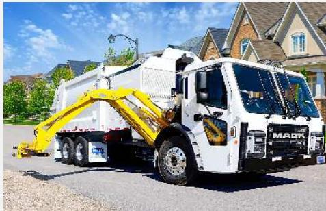
**Joystick Cab Controls:** reliable, ergonomic joystick controls deliver smoother performance and enhance usability. With the standard AutoLoad system, the operator can reach, grab, lift, dump, and return the arm to the stowed position using only the joystick and 2 buttons.
