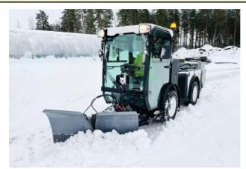
**CV Model** is a versatile, sustainable compact sweeper; ideal for municipal street cleaning, bike path maintenance, and year-around tasks. This machine supports a wide range of attachments for sweeping, pressure washing and snow removal. Also advanced features include rear rails for a drop spreader, and water nozzle connections for scrubbers or watering arms.
