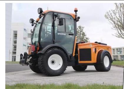
**MXC Model** is a great compact vehicle for urban maintenance – with a 130HP Engine, it can remove snow and ice from sidewalks and narrow pathways – then change to a sweeper outside of the winter season.
